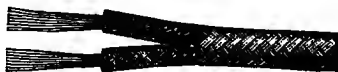
FIG. 65.—The cord of a telephone receiver. It consists of two strands of braided tinsel, insulated, and enclosed in a woven sheath. A metal pin is secured to the end of each strand, and this is inserted in the grooves of the binding-post to give electrical connection.
